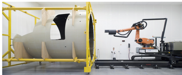
图4 大型复杂复合材料构件的激光超声检测 Fig.4 Laser ultrasonic NDT for composite component
